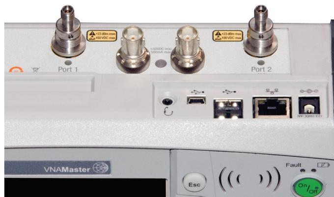
Optional K(f) test port connectors are available for precision measurements to 20 GHz.
